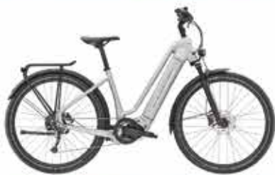
Trek Allant+ 7 Lowstep 5 Matte Quicksilver Motor Bosch 85 Nm, Akku 500 Wh
